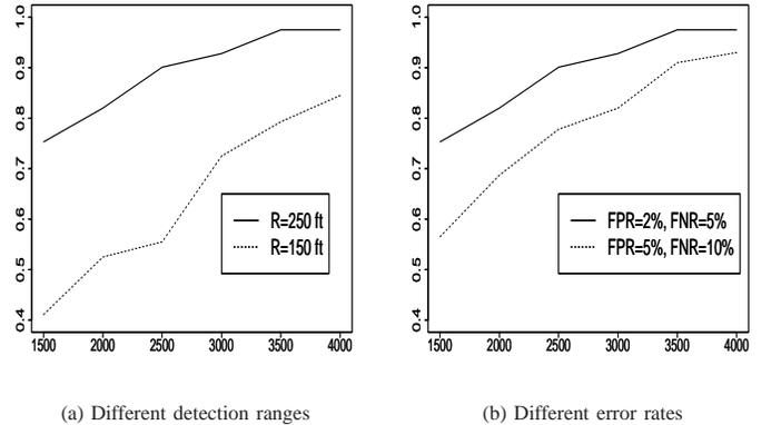
Fig. 2. Detection Power Comparison: (a) Two different sensor ranges with the same error rates (2%, 5%). (b) Two different sets of error rates with the same sensor range of 250 ft. The horizontal axis is the number of sensors.
