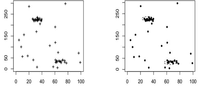
Fig. 1. Cluster detection. The left plot displays positive signals from the sensors via simulation. The right plot gives the detected clusters representing two nuclear sources.
