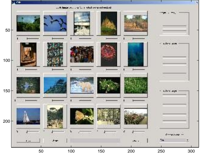
Fig. 1. Interface of the Content-based Image Retrieval System. The lower-left button is for randomly displaying and browsing images. Sliders are used to specify query image.
